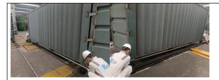
3. The 2nd shot blasting and paint application process commenced this afternoon, checked the condition on site, found the poor 2nd shot blasting on the interior corner post hidden area, rectified on site, condition improved later. Detail as below:
